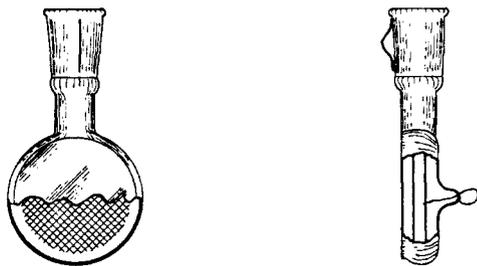
Figure 5. Electrochemiluminescence cell employed in the integrating-sphere studies.
